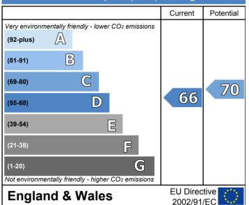
The environmental impact rating is a measure of this home's impact on the environment in terms of Carbon Dioxide (CO<sub>2</sub>) emissions. The higher the rating the less impact it has on the environment.
