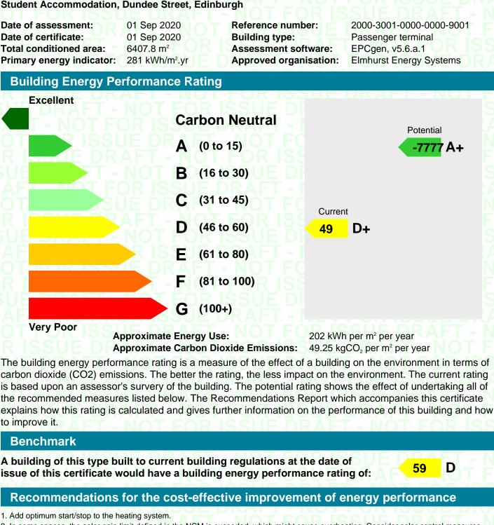
2. In some spaces, the solar gain limit defined in the NCM is exceeded, which might cause overheating. Consider solar control measures such as the application of reflective coating or shading devices to windows.
